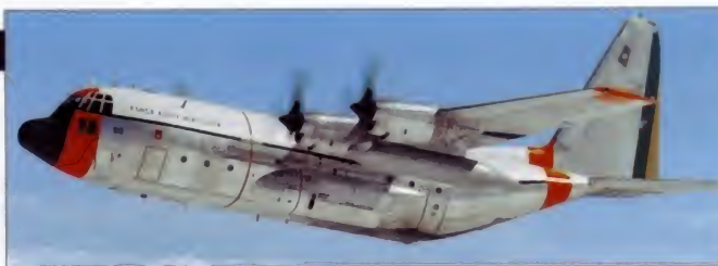
Left: External fuel tanks located between the engines were an identifying feature of the C-130E.
